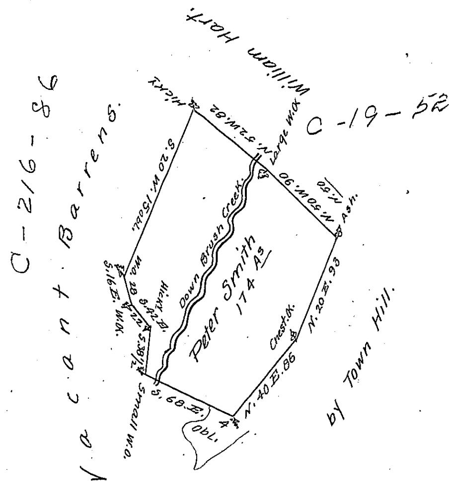
A Draught of a Tract of Land called the Cave Spring Situate on the S.W. Branch of Brush Creek about three Miles above the Gap, adjoining a Survey said to be made for William Hart in Colerain Township in the County of Bedford containing one hundred and Seventy four Acres and the usual Allowance of six P. cent for Roads &c. Surveyed the first Day of September 1774 for Peter Smith in pursuance of a Warrant dated the first day of July 1774 by
